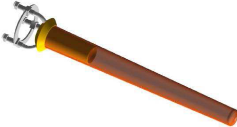
Figure 2.5: The 40 cm long cylindrical Kapton target cell used for the g12 run. (Image source: [4])
